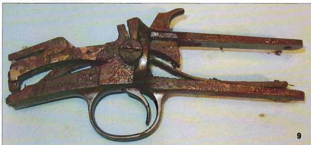
This is the time to check on the condition of the springs. Some guns have a mess of springs; coils, flat, round, some have few. We are looking for a loss of temper, springiness if you will. Can you easily bend a stiff flat spring, will a coil spring compress and rebound properly, same with round wire hairpin springs? If you find a suspect spring, where did it come from, large or small spring, just that one or others in the same gun?
