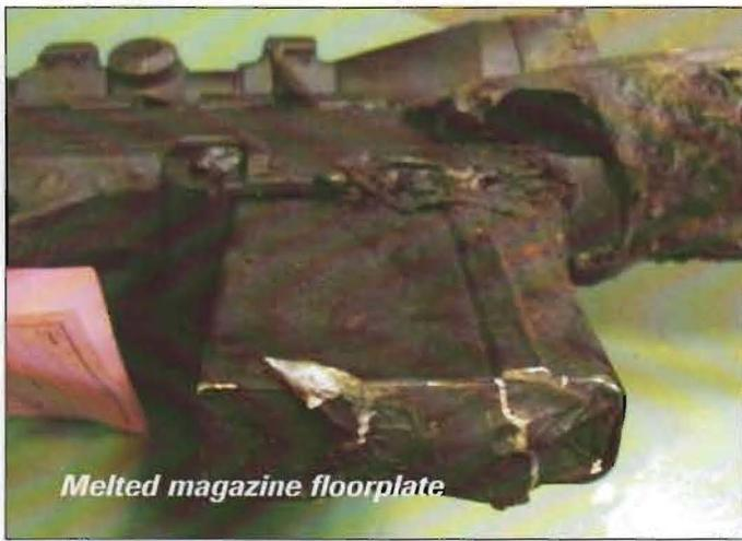
*Melted magazine floorplate*
