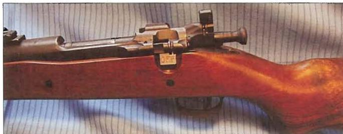
*Magazine cut-off switch in "Off" position*
